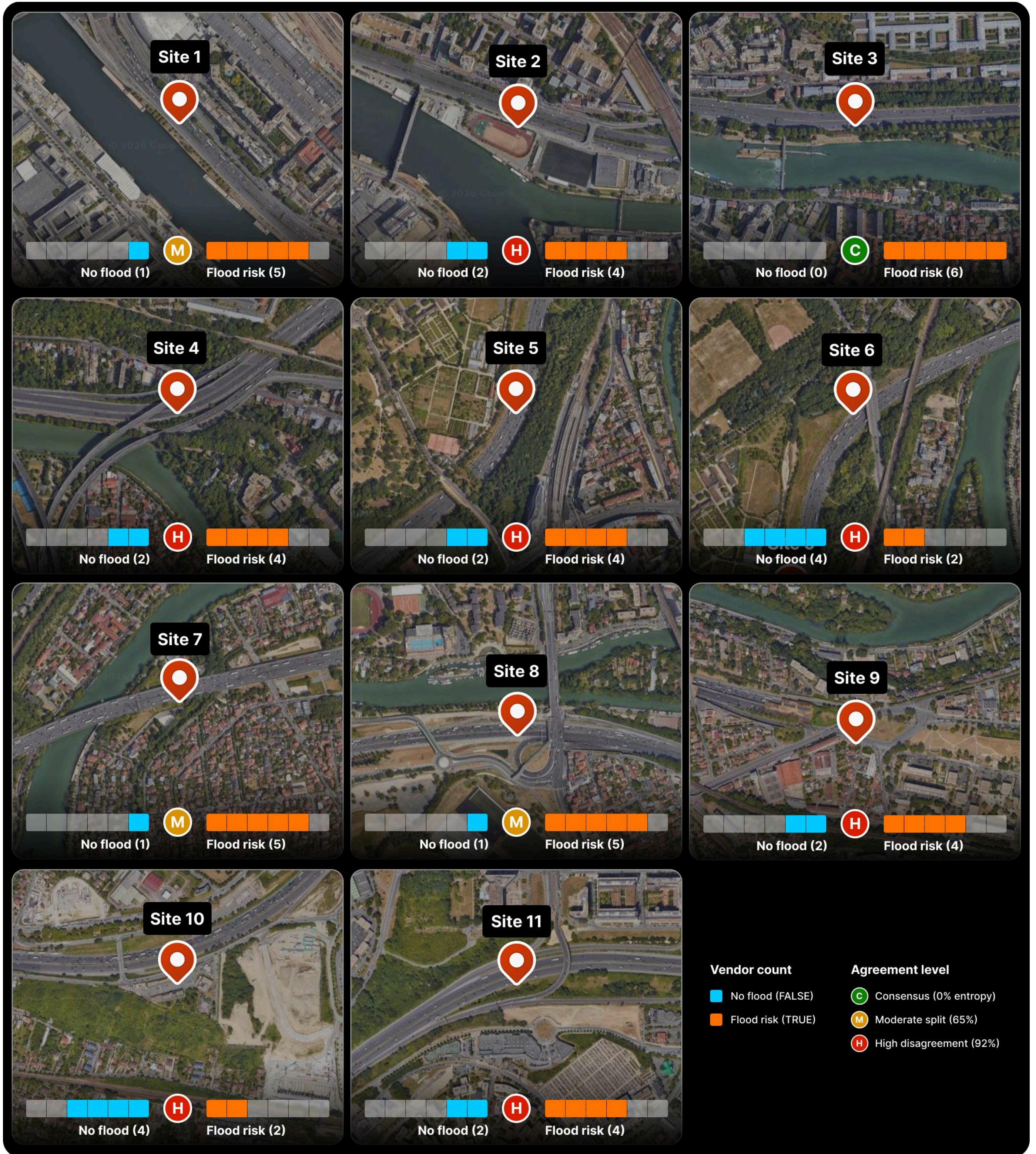
Figure 3-2. Count of vendors that indicate flood risk (blue = no flood, red > 0 millimeters inundation) across 11 sites of the A4 toll road near Paris. Riverine and rainfall-based flooding were considered.
